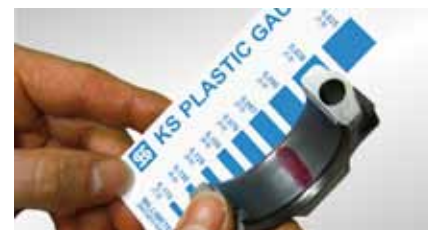
Checking the plain bearing with “KS Plastic Gauge”
