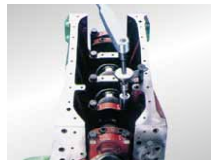
Checking the plain bearing with “KS Plastic Gauge”
