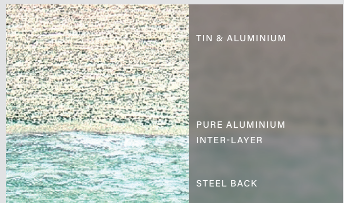
[FIG.32] Cross-sectional cut through a bearing shell made of A370°. The pure aluminium inter-layer bonds the tin-aluminium onto the steel back.
