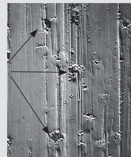
[fig.18] 300 times magnified view of the surface of a crankshaft journal made of nodular graphite iron after grinding. One can clearly see the lids explained in figure 17.
