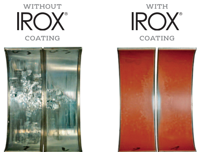
Bearing shells lined with the A-650 Al alloy substrate after endurance testing on a rig with 80 MPa for 250 h
