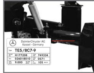
New identification plate can be found in the centre of the axle housing
