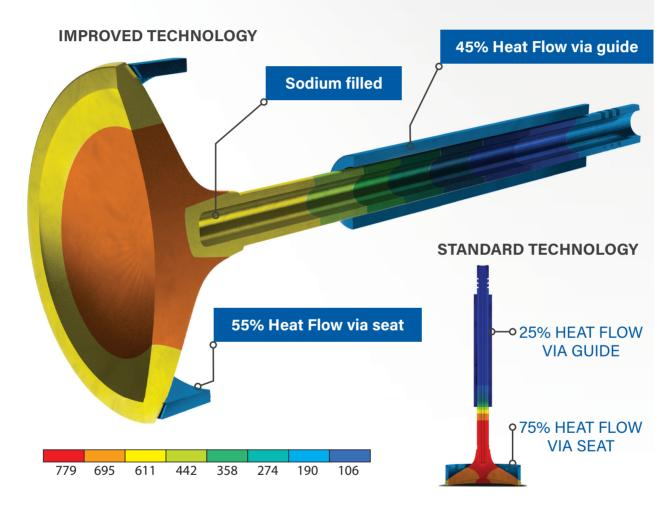
The heat dissipation via the valve guide is improved with sodium-filled valves, which helps to increase durability of the valve. Its hollow structure makes the valve lighter and helps reduce automotive emissions.
